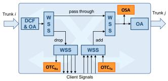
Fig. 1. Simplified optical node architecture with OTC and OSA monitoring systems
