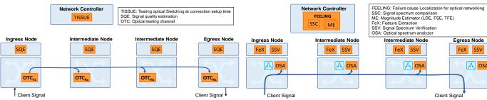
Fig. 2. OTC active monitoring for commissioning testing and failure localization
