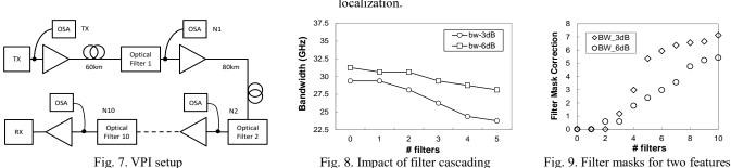
Finally, the DP-QPSK signal ends in a coherent receiver that compensates for the impairments introduced throughout the transmission. Emulating the optical node architecture in Fig. 1, coarse-granular OSAs are placed after every filter to analyze the optical spectrum. OSAs have been configured with a granularity of 625 MHz, i.e., every 37.5 GHz frequency slot is represented by 60 < f, p > pairs.
